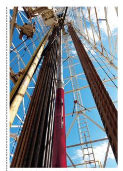
The Endura dual-string section mill creates a stable, permanent, and verifiable rock-to-rock barrier, cutting the P&A rig time in half. The barrier seals across the borehole by milling both inner and outer strings and mimics natural bedding.
