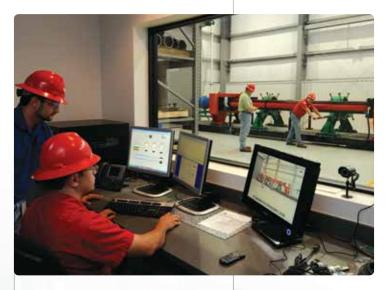
Unlike conventional testing of expandable connections, the DLX simulator can uniquely and accurately replicate downhole conditions that the expanding casing experiences in a real well environment.
