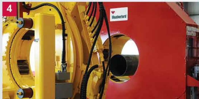
4 Pipes are positioned in the ComCAM bucking unit and made up to the torque specified in the TPC system, which also records the makeup data.
