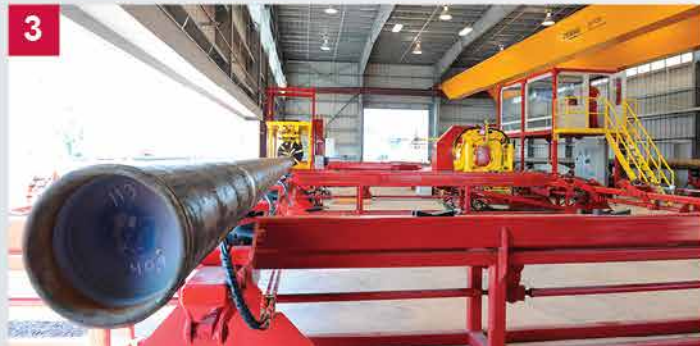
3 The walking tables transport the pipes to the ComCAM line conveyor.
