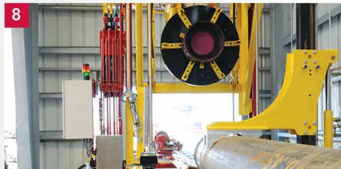
8 Thread protectors are removed from each end of the made-up stand by the automated thread-protector remover.
