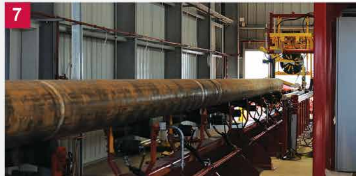
7 The stand is rolled over to the hands-free, drift-line conveyor, which transports it back inside the facility to the lance-drift/length-measurement station.
