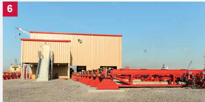
6 The ComCAM line conveyor transports the made-up stand out of the facility.
