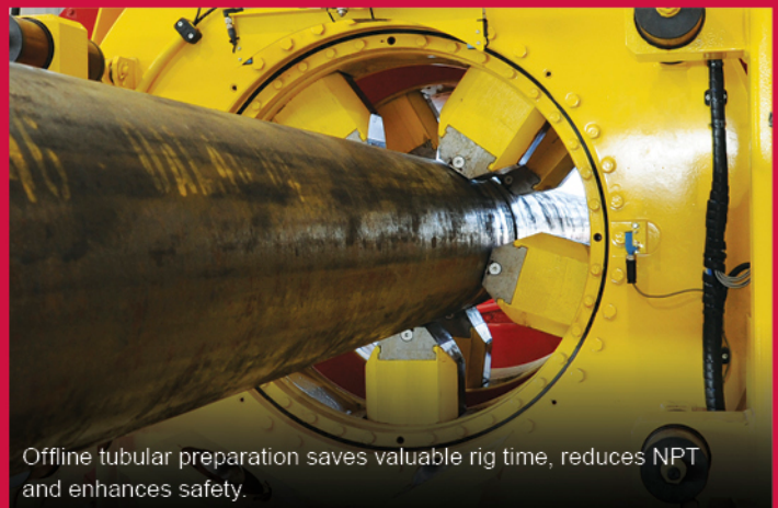
Nonmarking jaws enable makeup of premium pipe without undesirable grip marks.
