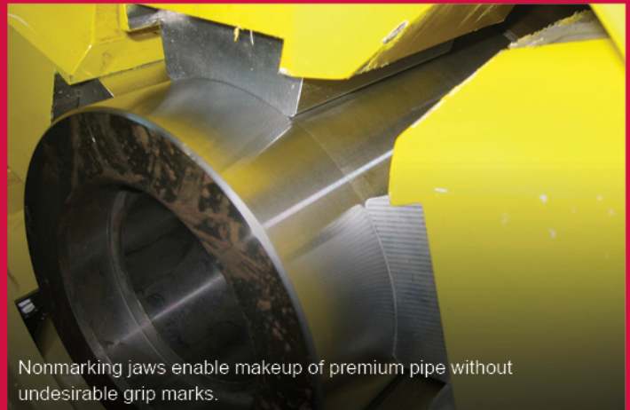
4 1/2-in. to 26-in., 200,000-lbf-ft bucking unit.
