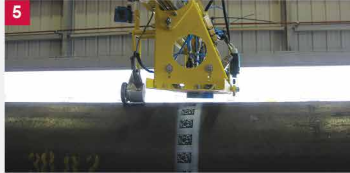
5 The stand ID assigned to the stand in the TPC system, is printed on the pipe as a 2D Data Matrix code.
