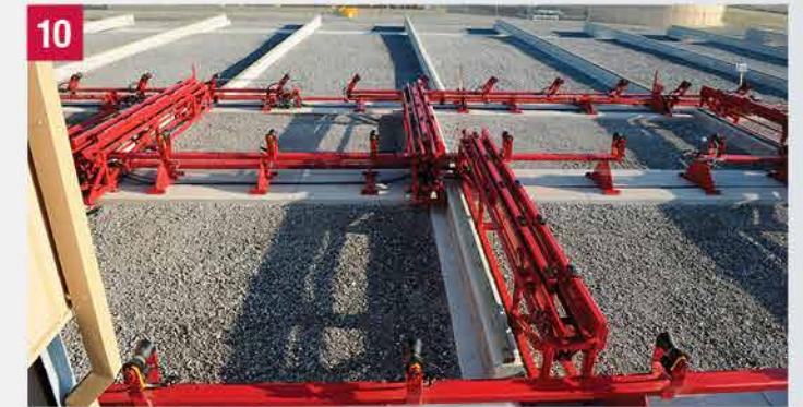
10 The drift-line conveyor transports the stand out of the facility and over to the stand conveyor for storage until ready to ship.
