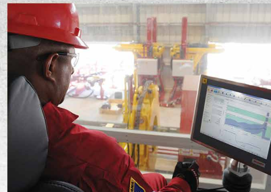
The automated bucking facility is run by a highly trained, pipe-handling specialist who directs the entire mechanized operation from the safety of a state-of-the-art control cabin.
