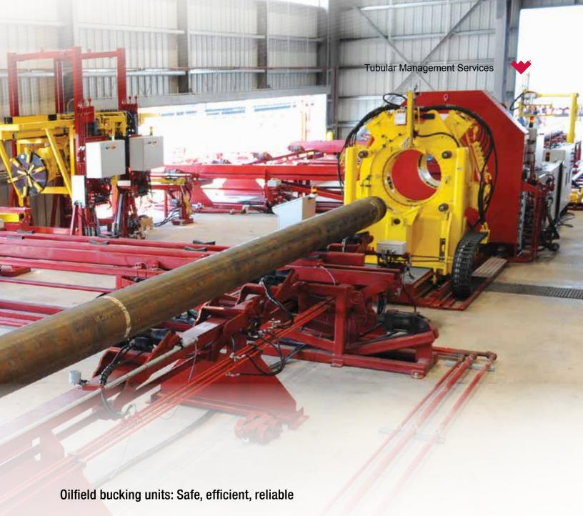
Off-site handling and bucking systems and torque/turn recording systems enable makeup and breakout of API and premium-thread tubing, casing and drillpipe in double or triple lengths.
