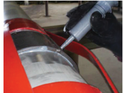
PoxiLok epoxy-injected stop collar
