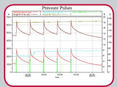
Figure 8: ACTiFRAC pulses to trigger delayed opening of ARID 3
