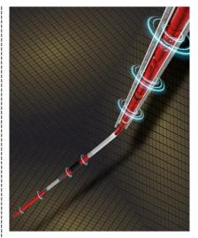
The world's first and only remote-activated installation system delivers upper and lower completions in a single trip.
