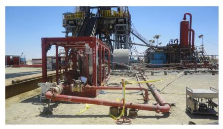
Used for the first time in an onshore well in Egypt, the Weatherford MPD control system enabled managed pressure drilling and managed pressure cementing operations.
