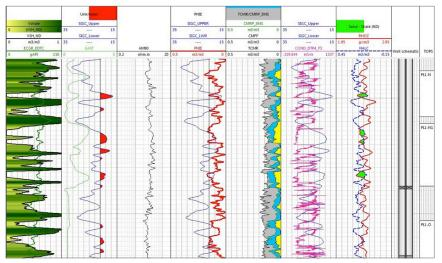
The Weatherford Raptor 2.0 cased-hole evaluation system gathered data showing clear gas-bearing sandstones (marked in red)
