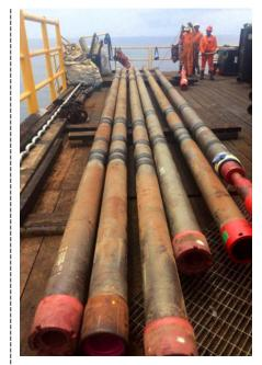
Weatherford used 225 ft (68 m) of MetalSkin cased-hole liner to isolate unwanted perforations and damaged casing, which stopped water production and improved well performance.
