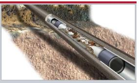
Weatherford's *MetalSkin* cased-hole liner system permanently and cost-effectively repaired the corroded casing, provided the optimum hole size, and restored the pressure integrity of the casing in three separate wells.
