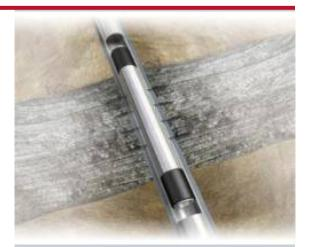
Weatherford's *MetalSkin* expandable cased-hole liner system repaired an interval of corroded casing with a permanent, cost-effective solution that provided the maximum hole size as compared to a conventional liner, facilitating continued production and future well work
