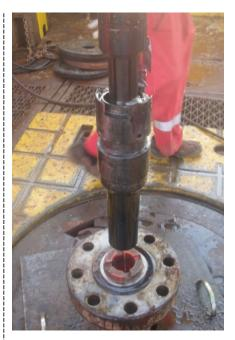
A Weatherford thru-tubing fishing services team retrieved a PX plug that was stuck downhole. This success eliminated the need for a costly recompletion operation and saved the operator 7 to 8 days of rig time.
