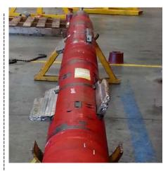
The Endura DSSM features specially designed blades and stabilizers that provide two points of stabilization while creating finer, more manageable cuttings.
