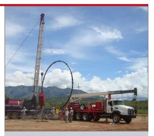
*COROD* continuous rod's uniform contact loading is the key to improving production performance in highly deviated wells. The uniform body design provides an even distribution of contact loads, leading to a significant reduction of wear-related problems on the rod string.
