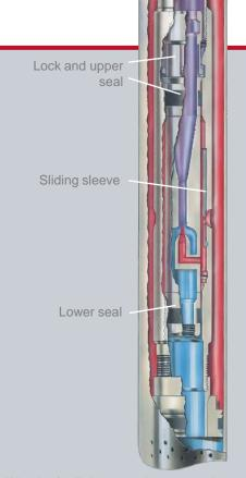
Weatherford's jet pump has no moving parts. Its pumping action is achieved through energy transfer between two moving streams of fluid, greatly reducing the risk of failure sometimes associated with other forms of lift.
