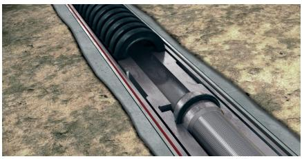
The patented design of the STP reduces sand damage by moving sand upward through the pump and away from the barrel/plunger interface.
