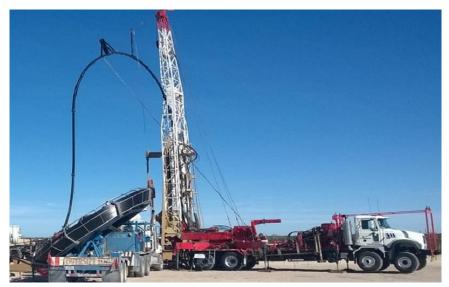
A Permian Basin operator replaced conventional guided sucker rods with Weatherford semi-elliptical COROD continuous rod for an 87% reduction in tubing leaks and 81% lower rod-string failure rate.
