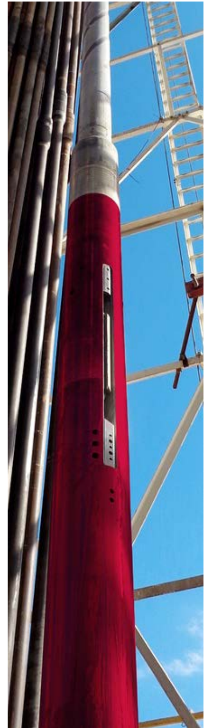
The Weatherford Endura DSSM mills inner and outer casing strings to efficiently prepare wellbores for cement plugging.
