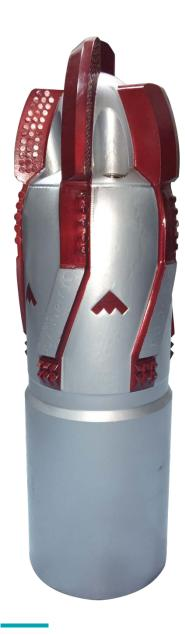
The CleanReam bit has a robust cutting structure that includes PDCs and a concentric nose dressed with TSP diamond cutters.
