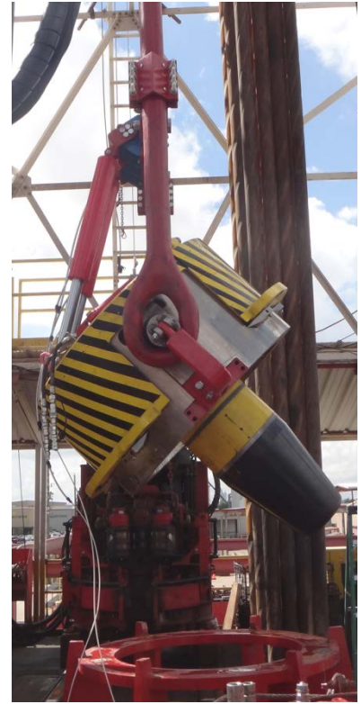
The DRE 500 enhances safety and efficiency when running flanged riser connections.
