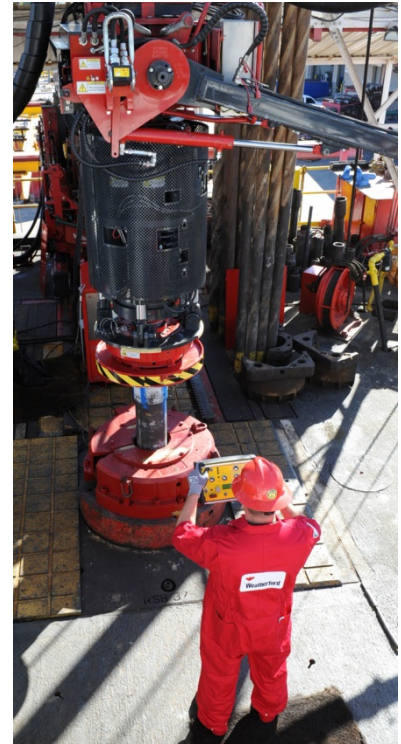
The TorkDrive EM tool directly integrates with existing rig control systems to enable operation from the driller's cabin, which reduces personnel on the rig floor.
