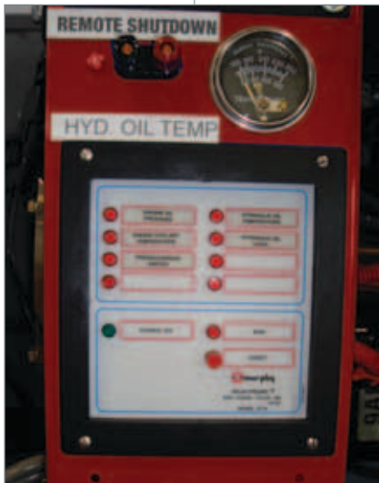
The ST8 shutdown control panel (optional) aids in troubleshooting the engine and hydraulics during a malfunction.
