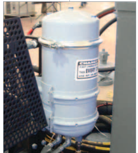
The Luberfiner filter (standard with GM models) improves the engine oil filtration process and aids in extending oil-change intervals, while also lowering annual maintenance costs.
