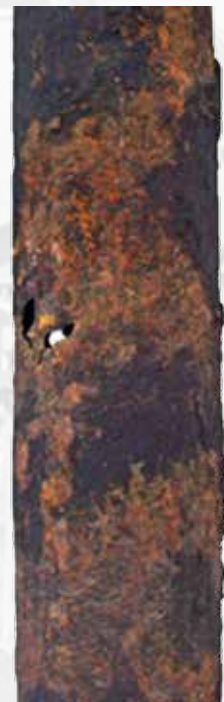
UltraView technology revealed the casing defects (left) in the actual pipe (right) that was pulled from the well
