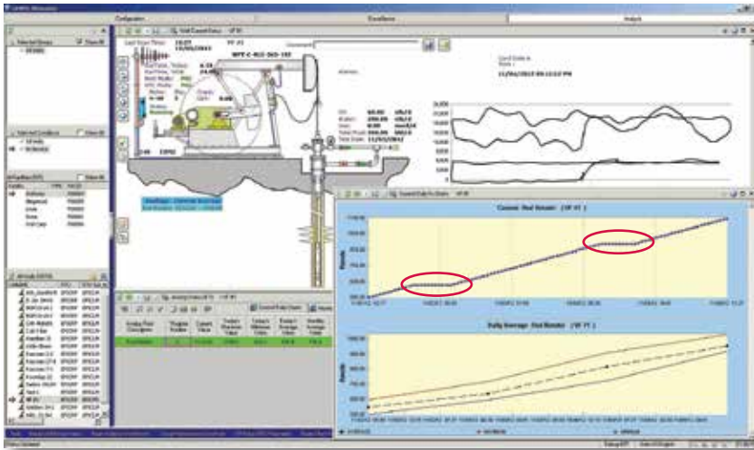
Screenshot of the intelligent rod rotator’s revolution counter being trended in the LOWIS™ software. The trend identifies two periods (circled in red) when the pump was running and the rotator was not working as expected. The condition generates an alarm signifying the need for attention or action.
