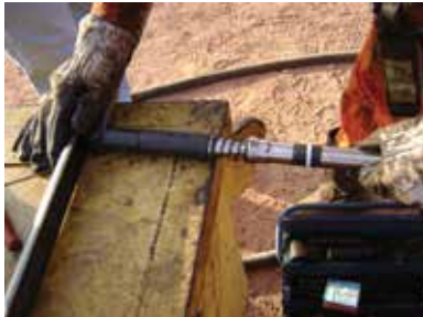
Waterflood valve inspected and prepared for assembly.
