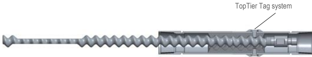
Fig. 6. TopTier tag system PC pump configuration.
