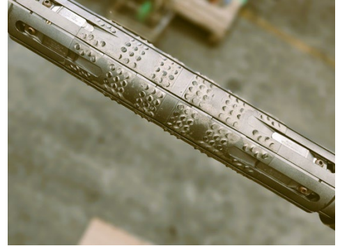
The slips of the Weatherford ISO Ultra Extreme bridge plug are capable of withstanding a differential of 15,000 psi (103.4 MPa).
