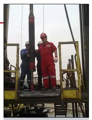
Weatherford's *IPP* packer provides a positive, pressure-tight seal for annular isolation between the workstring and casing or open hole to assist in remedial or abandonment applications during drilling and production. Compatible with drillpipe, threaded tubing, and coiled tubing, this packer offers the versatility of a temporary or permanent seal for single- or multiple-packer configurations in wells of any deviation.
