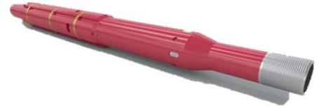
*The circulation valve (above) is a metal-to-metal sealing system that opens with pressure pulses and closes with RFID tags, eliminating surface control lines.*
