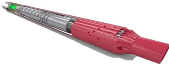
*The hydraulic power unit (HPU) shown above is a tubing-mounted, self-contained, remotely operated, multifunctional downhole unit that provides interventionless actuation of any hydraulically operated device, including actuation for packer setting, sleeve operation, and valve operation.*
