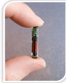
The Weatherford Keystone upper completion system (right) uses RFID tags (above) to enable entirely remote operation. The system isolates the reservoir, sets a production packer, opens a circulation valve, displaces the annulus and tubing to a lighter completion fluid, closes the circulation valve, pressure tests the tubing for integrity, and finally opens the isolation valve to bring on the well.
