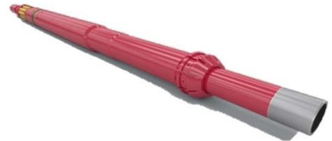
*The production packer (above) is equipped with a cut release zone for workover flexibility and is set with 4,000-psi (27.5-MPa) applied tubing pressure.*
