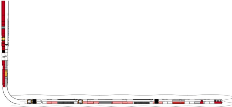
The tool string included (from top to bottom) a liner-top packer, an OptiSet FL valve, MORPHISIS annular swellable packers, MaxFlo screens with FloReg DA devices, an SCCV, and a FREGS.
