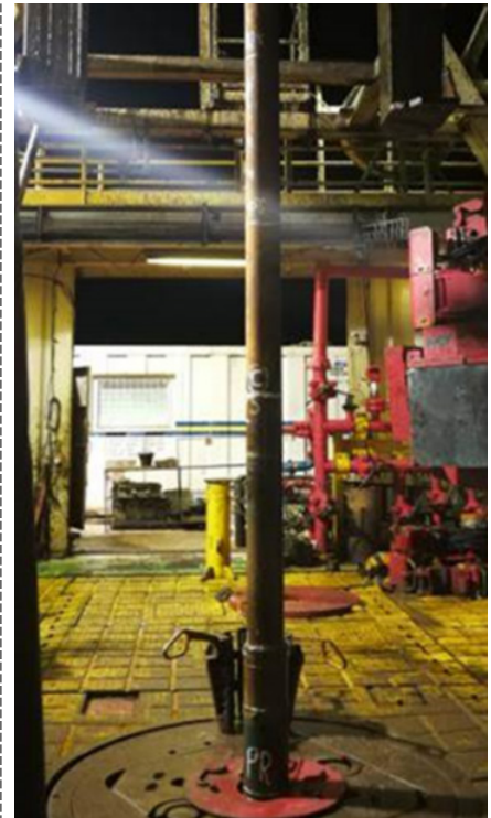
Weatherford crews made up the WFX0 completion equipment, shown ready to run in the hole.
