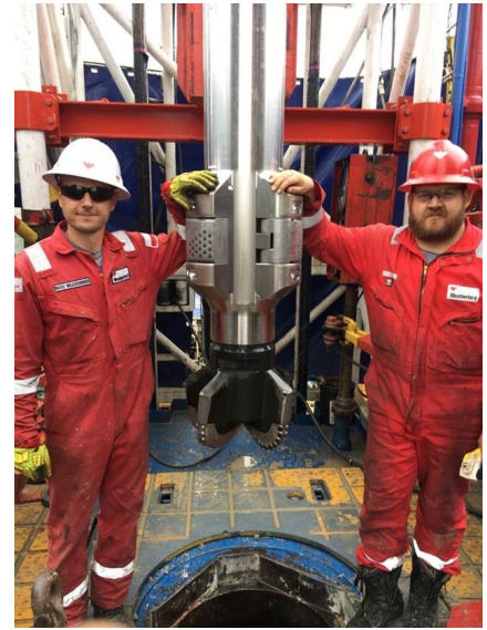
The Magnus RSS 1100 drilled the 17 1/2-in. hole section of an onshore, vertical well faster than planned.
