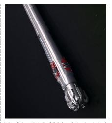
Unique features-including fully independent pad control and a true-inclination hold—make the Magnus RSS a complete package that helps operators stay on plan and reduce well construction costs
