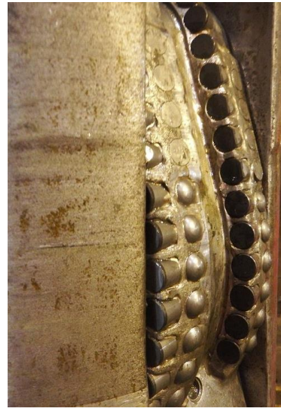
Upon retrieval to surface, the cutters on the RipTide RFID underreamer showed only minor wear.
