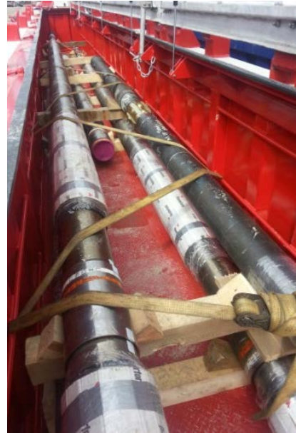
The liner-hanger system provided reliable liner-top isolation, reached a 23,225-ft (7,079-m) depth, and enabled rotation during cementing operations.
