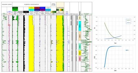
Composite log with the information obtained: GR-DEN-NEU, elemental concentration, well schematic (to see double liner and liner change) with the re-entry perforated open intervals, mineralogy, porosity, and oil saturation. Integrated with field generic fractional flow curves from relative permeabilities to understood high BSW in production.
