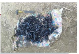
In most heavy-oil fields in Venezuela, using PCPs results in elastomer gum debris and sand buildup on the liner that create obstructions and interrupt production. In these four wells, the Cyclone Bailer tool and CT services removed the obstructions in a quick and cost-effective manner and fully restored production to previous levels.
