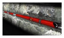
The Weatherford WidePak straddle system is a highpressure packer used for temporary or permanent isolation of tubing sections, perforations, or windows. Its large packer throughbore is set in one run using slickline and enables maximum production after setting as well as many intervention operations.
