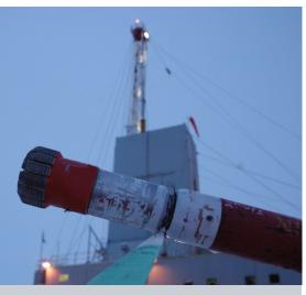
In combination with the CCMP mill, the e-CTD motor (shown above) drilled out 14 frac sleeves and 14 balls in one 3-hour trip. Because the motor did not have to be changed mid-operation, the operator saved significant rig time and costs.
