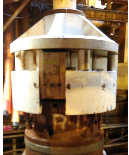
The top image shows the MOST Plus system, a proven subsea wellhead recovery tool that latches onto the external profile of a subsea wellhead while a hydraulic internal casing cutter cuts the conductors. The bottom image shows a well conductor cut by this system and then recovered.
