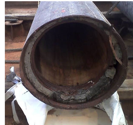
The top image shows the MOST Plus system, a proven subsea wellhead recovery tool that latches onto the external profile of a subsea wellhead while a hydraulic internal casing cutter cuts the conductors. The bottom image shows a well conductor cut by this system and then recovered.
