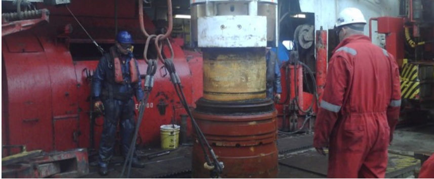
Weatherford used a number of customized and proprietary tools, including the M.O.S.T. Plus tool, to safely abandon 32 North Sea wells.
