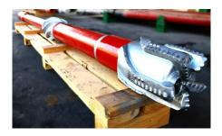
The AlphaST openhole PDC drill bit, coupled with flex mill facilitates quick departures in highly compressive formations, eliminating the need for time-drilling. The AlphaST features a hydraulic anchor which provides two independent, anchor-slip sections. These enable six points of contact against the formation to securely anchor the whipstock.
