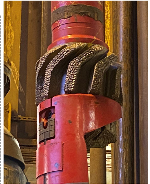
The exclusive HMR (Hydraulic Mill Release) system on the AlphaV eliminates the need for a traditional shear bolt.
