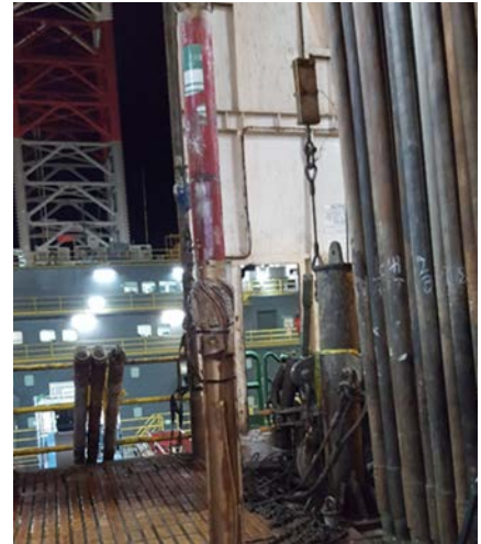
Using the shallow-angle QuickCut system, a Weatherford casing exit team milled through three concentric casing strings in a single trip with no remedial work required.
