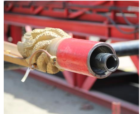
Shallow Angle QuickCut lead mill with patented AccuSet 2.0 sleeve being installed prior to deployment.
