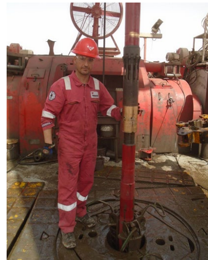
The Weatherford collapsible landing sub is rigged up and ready to run in the hole.
