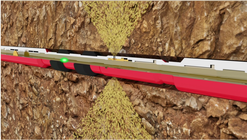
An RFID tag (green) is pumped downhole to transmit commands to stimulation tools.
