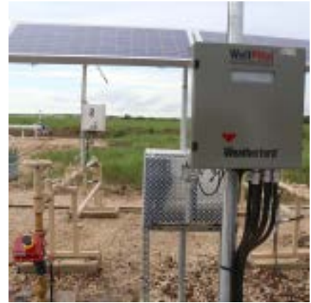
The above photo shows the WellPilot controller with injection-gas control valves and solar panels in the background.
