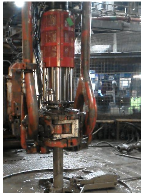
The FlowMaster tool extended sealing around the tool joint.
